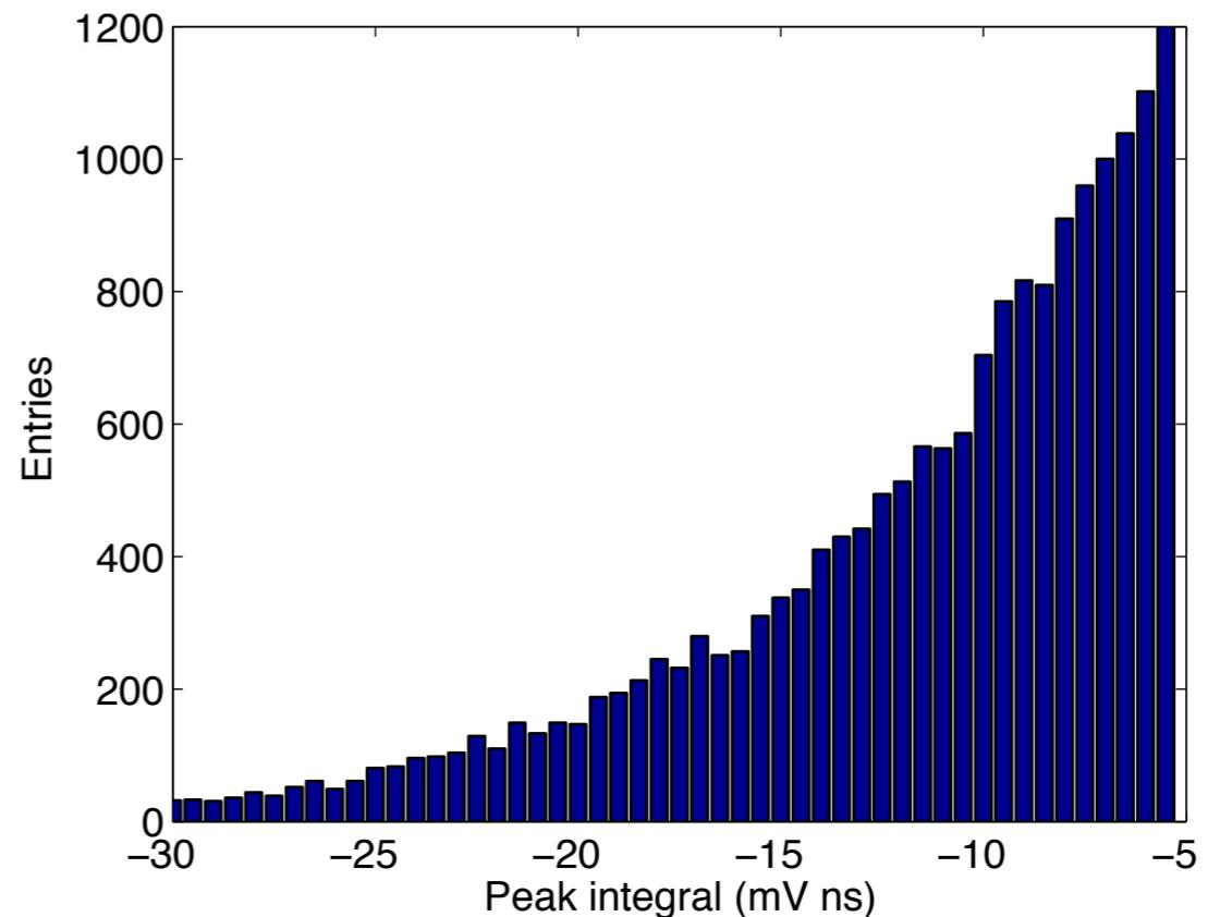
According to the calibration, 24 MeV gammas deposit 3.4 mV.ns with a peak of 0.7 mV.
