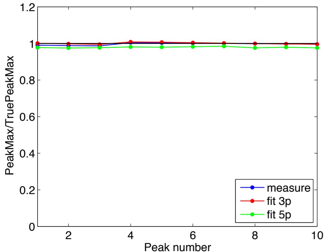
The results of the fitting are better, but the results for the directly measured value of the intensity maximum are already very accurate.
