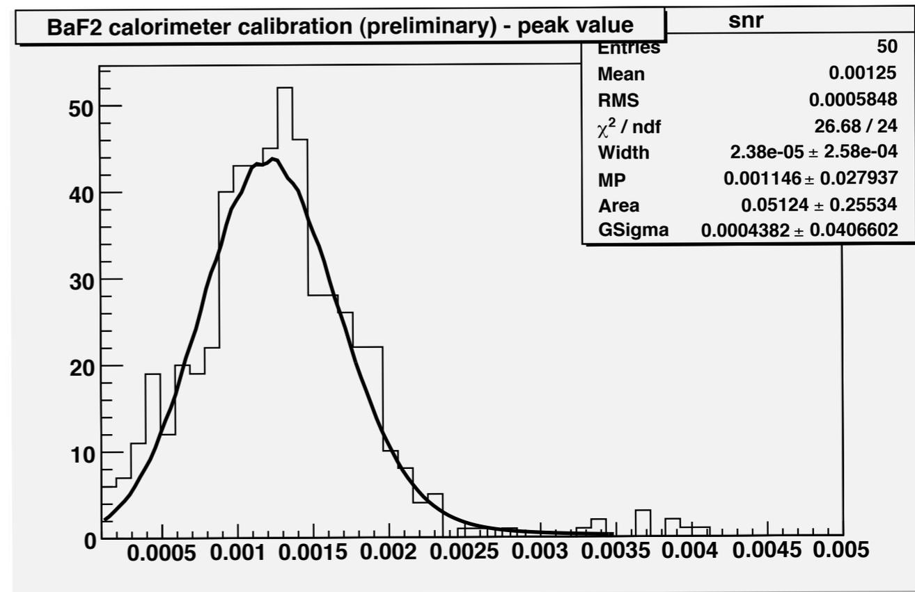
The most probable value for the integrated signal is 5.2 mV.ns and most probable value for the peak is 1.1 mV
