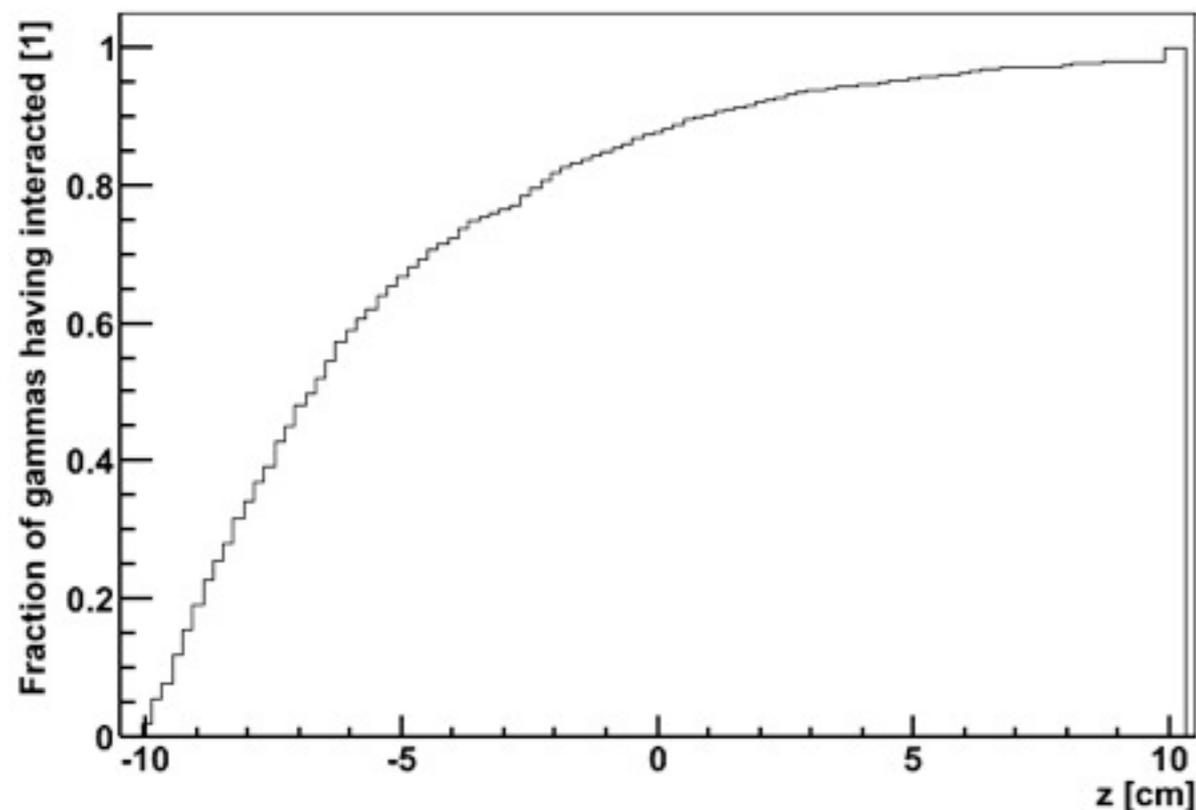
The high energy Compton gammas interact along the crystal while some of them pass the calorimeter without interacting.
