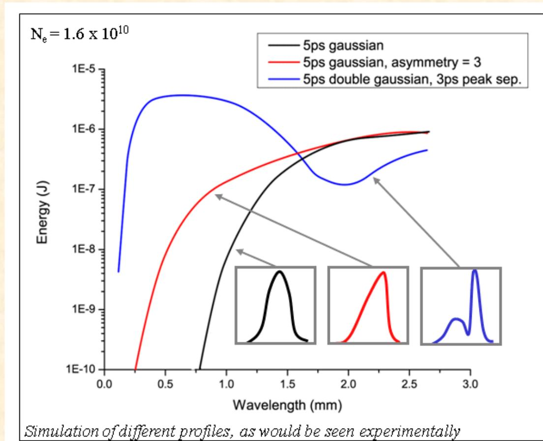
Different bunch profiles will give different radiation spectrums which can be reconstructed.
