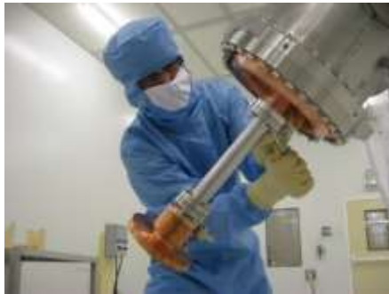
Assembling of coupler on the cavity
