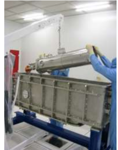
Cavity implantation in the vacuum chamber in the clean room
