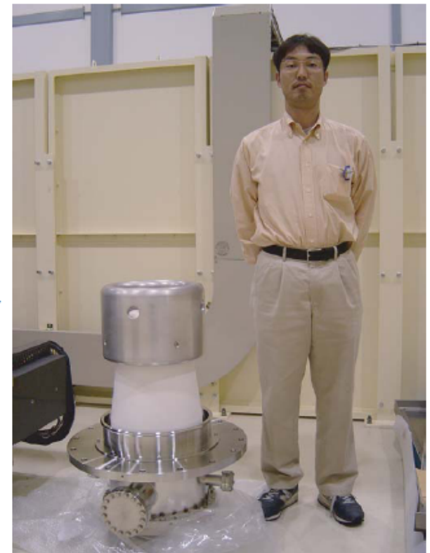
Spring 8 SCSS thermionic gun. (images source: T. Shintake, Spring-8) 40
