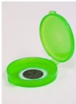
Exposed stretched Teflon filter, optimised for IBA analysis.
