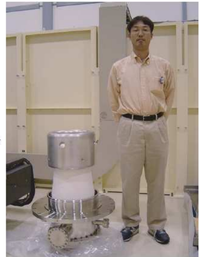
Spring 8 SCSS thermionic gun.
